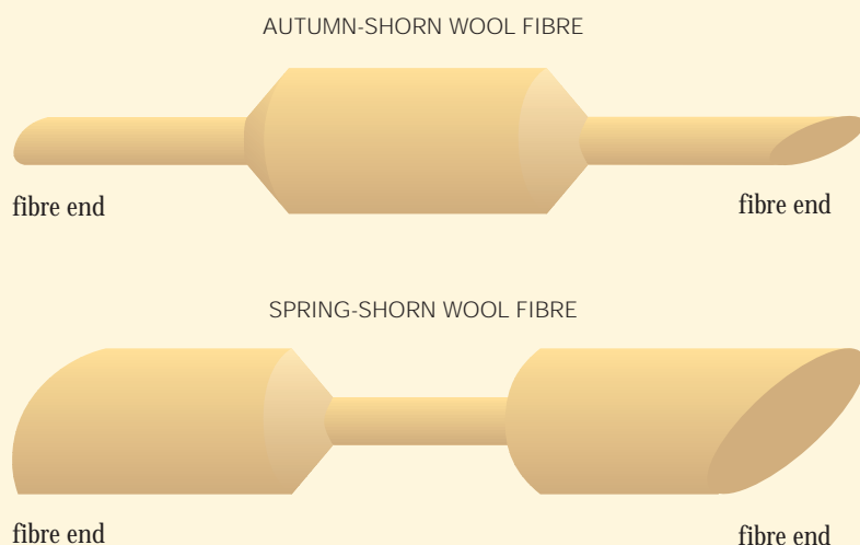
Figure 1 Effect of time of shearing on the fibre diameter profile of wools from Western Australia
