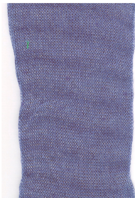
Illustration of unlevelness due to channelling during package dyeing.
