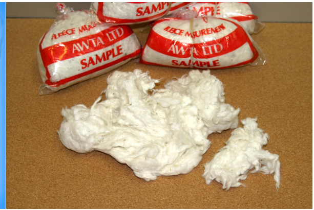
Scoured core samples
