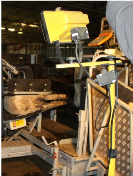
568 Figure 2. Sheep restrained in lateral recumbency using an electronic sheep 569 handler (Hdale Engineering Ltd, Auto Weigh Sheep Handler Model no: CWC 570 RC) for breech parameter scoring.
