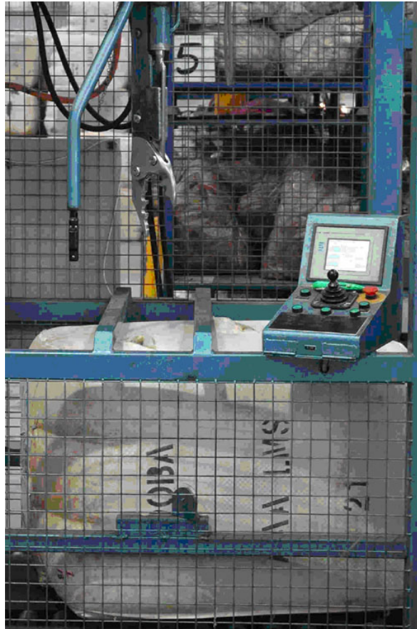
Figure 7.3 Grab machine with bale in place ready for sampling. Source: AWTA, (2005).
