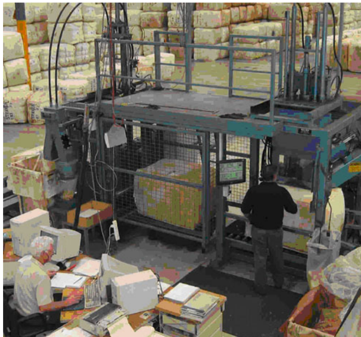
Figure 7.1 Sampling machine comprising a grab station on the right, bale weighing platform in the centre and core chamber on the left (mostly obscured by guarding).
