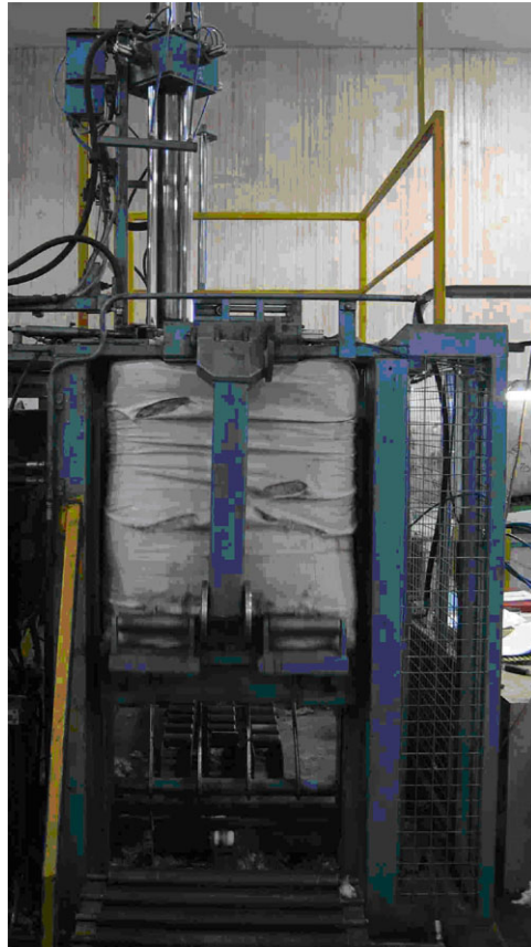
Figure 7.8 Core sampling a bale, bale is compressed against the roof of the chamber, core tubes penetrate from above. Source: Steere (2006).
