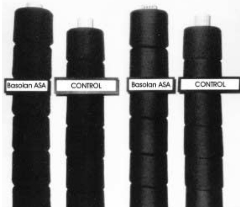
Effect of Basolan AS on the Bulk of Package-dyed Wool Yarns
