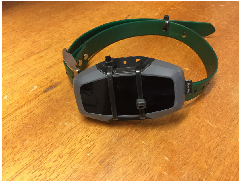
Figure 1.11: A prototype of an on-collar audio monitoring device, developed using a Thingsee [413].
