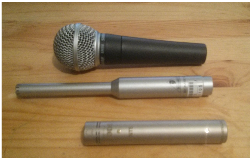
Figure 3.28: A comparison of microphone sizes. The top mic is the ubiquitous Shure SM58, the middle is a Behringer ECM8000 reference mic, and the bottom is the mic used in the system, a Rode NT5. Note the small size of the NT5.
