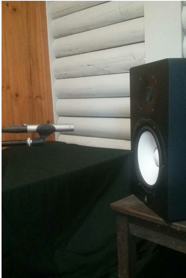
Figure 3.29: The standard testing set up used during experimentation. This image shows the microphone placed 20cm away from the sound source.
