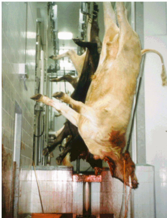
Figure 11.10. Low voltage stimulation being applied immediately post slaughter. Low voltage current being applied by nostril clamp and an anal probe. Notice the tetany of the front legs (compare with those of other carcasses). (Photo JM Thompson).
