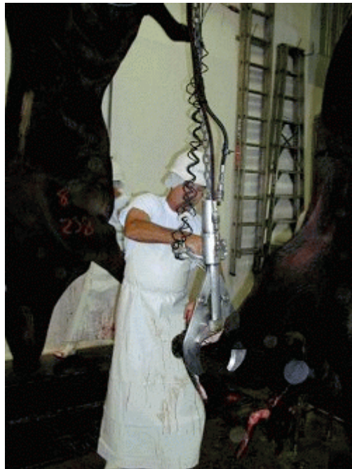
Figure 11.11. Using a pneumatic cutter to remove the feet (Photo JM Thompson).
