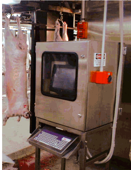
Figure 13.1 Lamb VIAScan being used to collect carcasses images which are then analysed and used to estimate carcass yield. Photograph supplied by J. Thompson.
