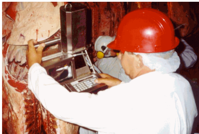
Figure 13.14. The video image chiller assessor capturing an image of the quartered site. Photograph supplied by J. Thompson.
