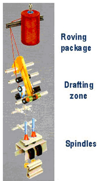
Figure 21.31 Worsted spinning. Source: Wood, Canesis Network Ltd (2007).
