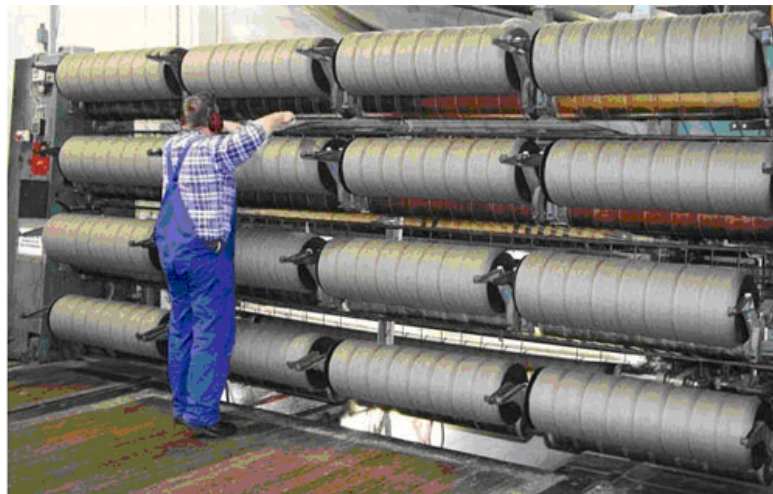
Figure 21.21 Condenser of woollen card showing the spools. Source: Photograph supplied by E. Wood, Canesis Network Ltd (2007).
