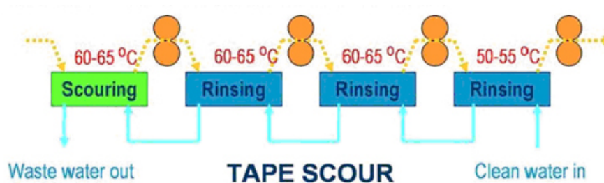
Figure 21.23 Tape scouring machine for woollen yarn. Source: Wood, Canesis Network Ltd (2007).
