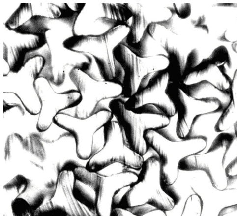
Figure 21.11 Trilobal cross-sectional shape of polyamide (nylon) fibres. Source: Image supplied by E. Wood, Canesis Network Ltd (2007).
