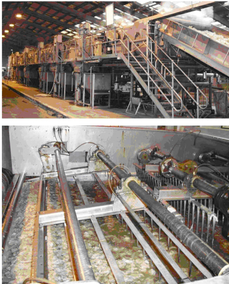
Figure 21.12 (a) a wool scouring line; (b) surface of a scouring bowl showing the rakes in action. Source: Photograph supplied by E. Wood, Canesis Network Ltd (2007).
