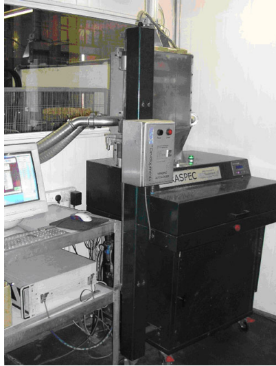
Figure 11.17 NiraSpec instrument in a wool scour, showing the sample delivery system and computer. Source: Wood (2006).
