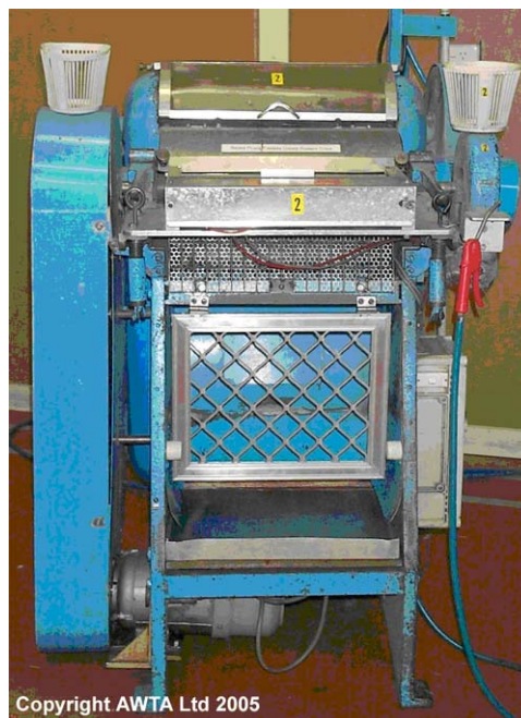
Figure 13.1 Shirley Analyser. Source: Fish, AWTA Ltd (2006) with permission
