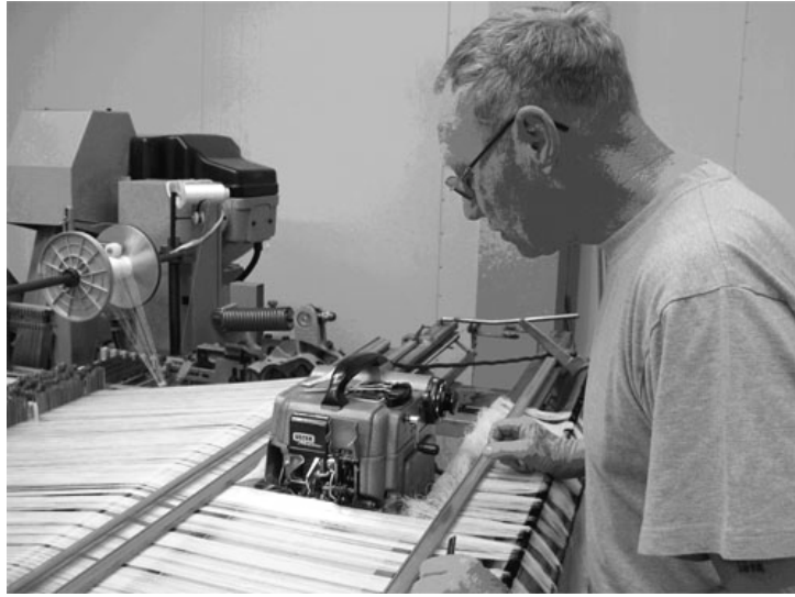
Figure 11.5 Use of a knotting machine to tie in warp yarns.
