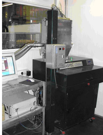
Figure 9.12 NiraSpec instrument in a wool scour, showing the sample delivery system and computer. Source: Wood (2006).
