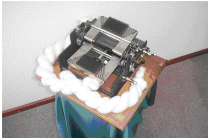
Figure 13.2b Schlumberger comb sorter. Source: Turk, J. (pers. comm. 2005).
