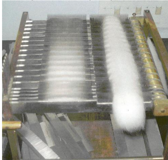
Figure 13.2a Suter comb sorter source. Source: Turk, J. (pers. comm. 2005).
