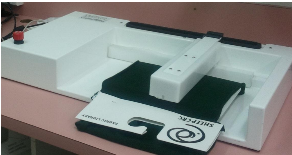
Figure 16.6: The Wool ComfortMeter with a fabric on the test bed.
