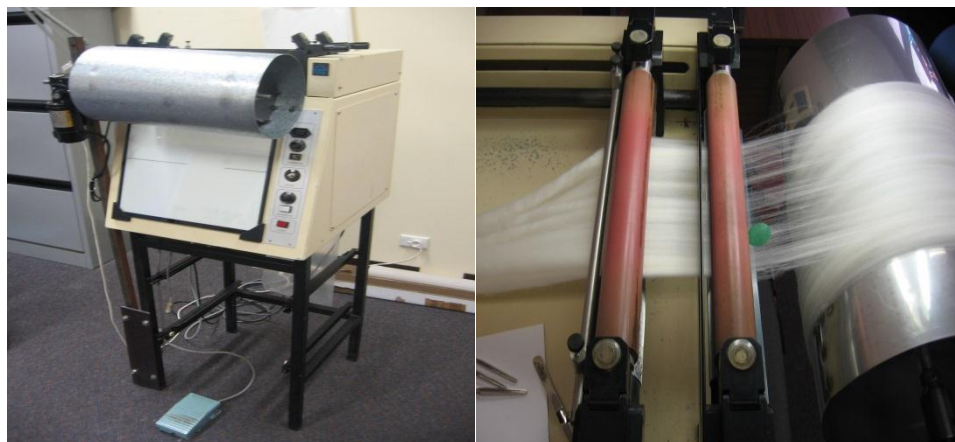
Figure 16.1: A Modified Toeniessen Drafting Machine
