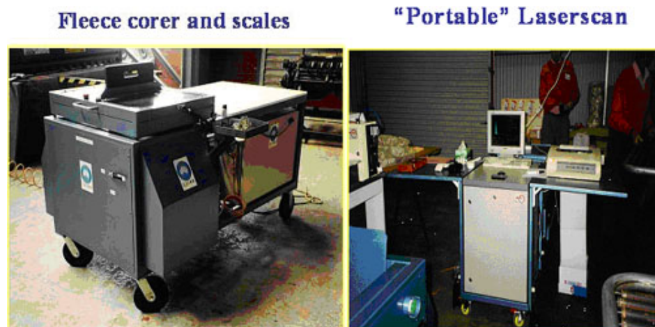
Figure 9.21 An image of a Fleecescan system showing the Coring, Snippet Washing and Fleece Weighing unit and the separate Laserscan section. Source: CSIRO Textile and Fibre Technology (pers. comm) with permission.
