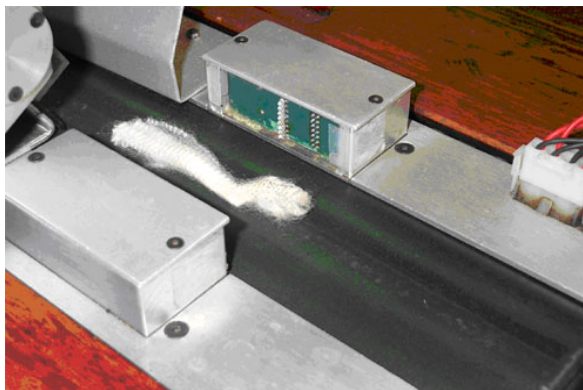
Figure 10.5 ATLAS staple length detector. Source: Crowe and Mahar AWTA (2006), with permission.
