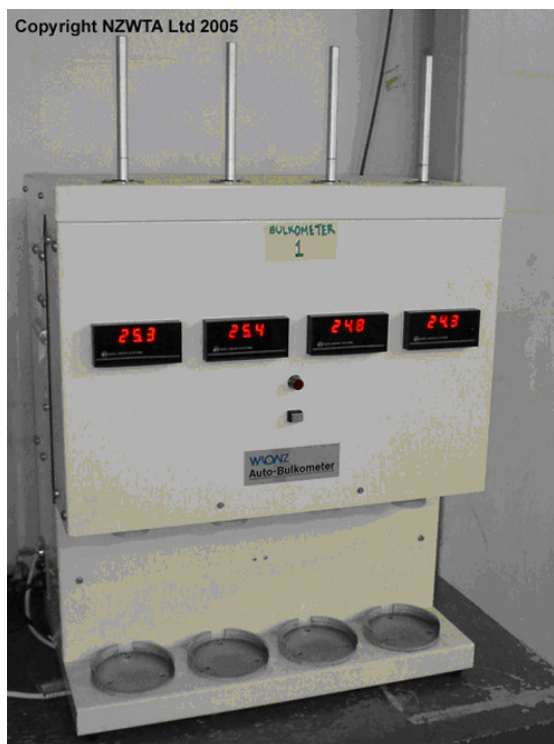
Figure 13.4 Auto-Bulkometer. Source: NZWTA Ltd. (2005) with permission.
