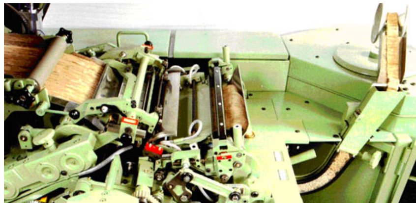
Figure 2.7 Combing machine. Source: NSC Schumberger.
