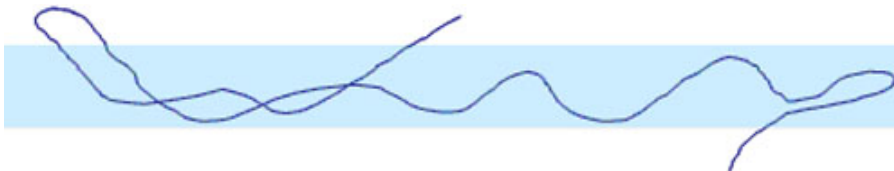
Figure 2.15 Typical fibre path in woollen yarn. Source: Wood, 2006.
