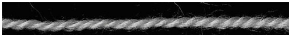
Figure 2.16 Two-fold woollen spun carpet yarn. Photograph supplied by E. Wood, courtesy Canesis Network Ltd.
