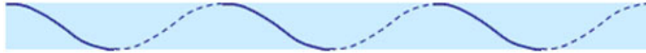
Figure 2.12 Helical path of a fibre in an ideal worsted yarn. Source: Wood, 2006.
