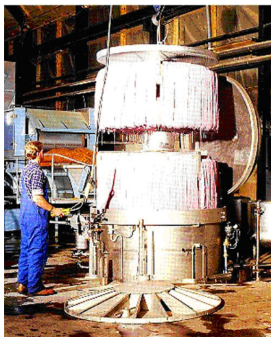
Figure 2.18 Hank dyeing machine. Photograph supplied by E. Wood, courtesy Canesis Network Ltd.
