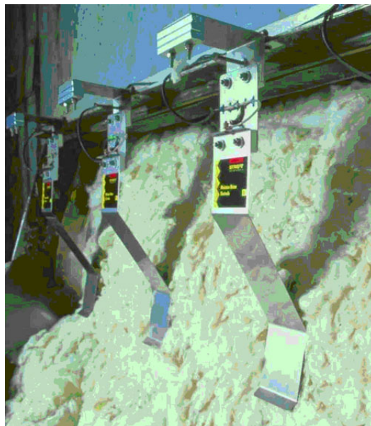
Figure 6.16 Drycom sensors for detecting the moisture content of dried scoured wool. Source: Streat Instruments.
