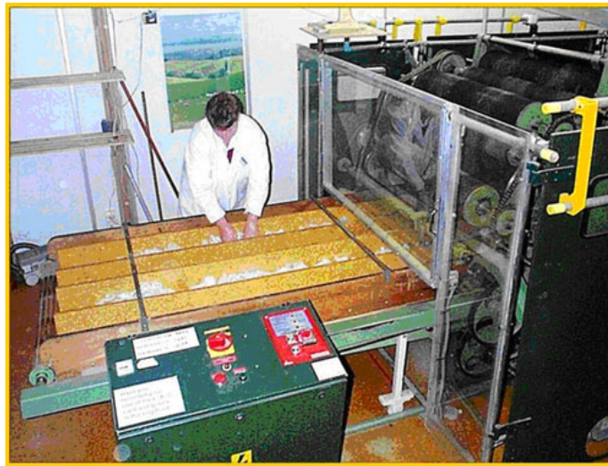
Figure 6.11 Carding step in LAC test showing the wool entering the machine. Source: Wood, 2006.
