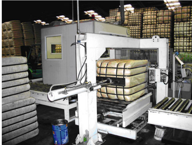
Figure 6.1 Core sampling in a woolscour. Source: Wood, 2006.
