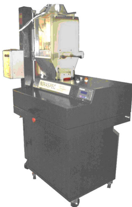
Figure 6.19 NIRASPEC S system for in-scour testing. Source: Wood, 2006.
