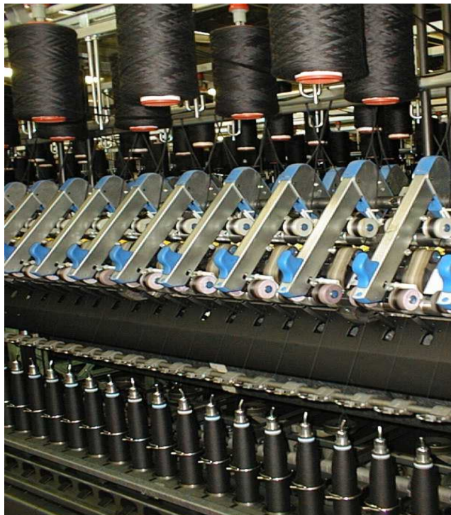
Figure 15.6 Partially collapsed (bent-finger) FP99/260 spinning frame. Source: Gaudino, Italy.
