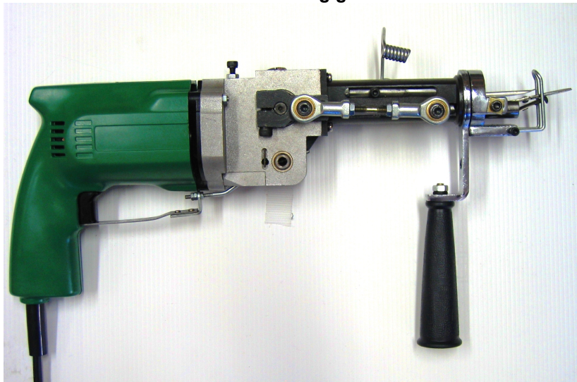
Figure 22.7 Mechanised hollow needle tufting gun. Source: Wools of New Zealand.
