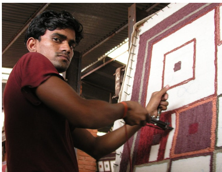
Figure 22.8 Hand tufting in an Indian carpet mill. Photograph supplied by E. Wood.
