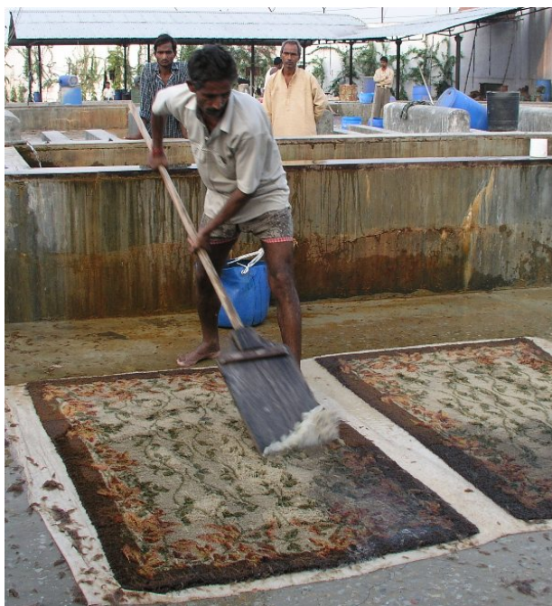
Figure 22.6 Washing of hand-knotted carpet in Indian carpet mill. Photograph supplied by E. Wood.
