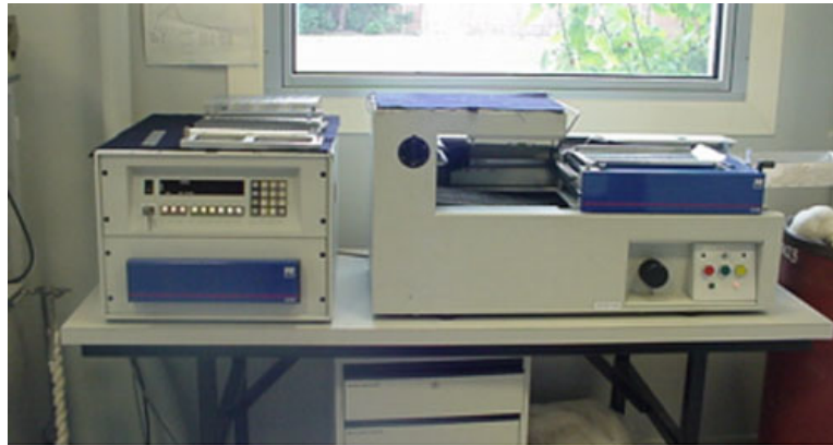
Figure 28.2 An Almeter measures mean fibre length and distribution. Source: CSIRO Textile and Fibre Technology (2005).
