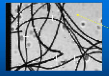
Measurement points are shown as lines crossing fibre
