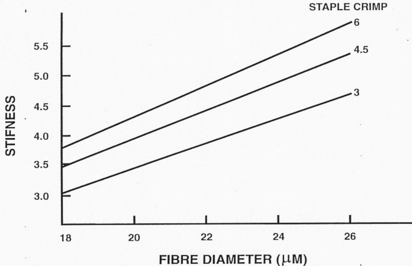
The effect of fibre diameter and staple crimp on
