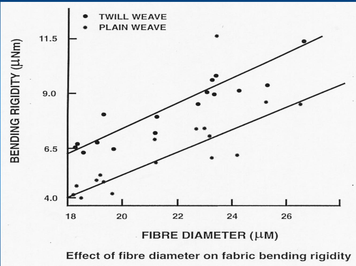
Effect of fibre diameter on fabric bending rigidity
